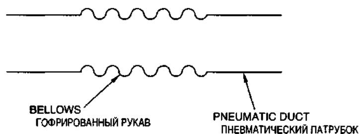
**BELLOWS (NO. 2)**, Corrugated folded or pleated container or compartment used to measure pressure.
