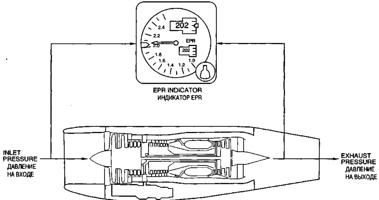
**EPR, SEE - ENGINE PRESSURE RATIO**
