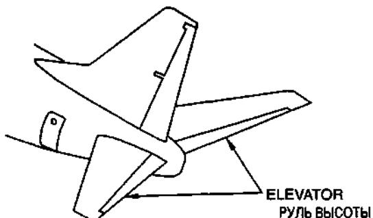
**EMPENNAGE**, The rear portion of an airplane consisting of fuselage, horizontal stabilizer and vertical stabilizer.
