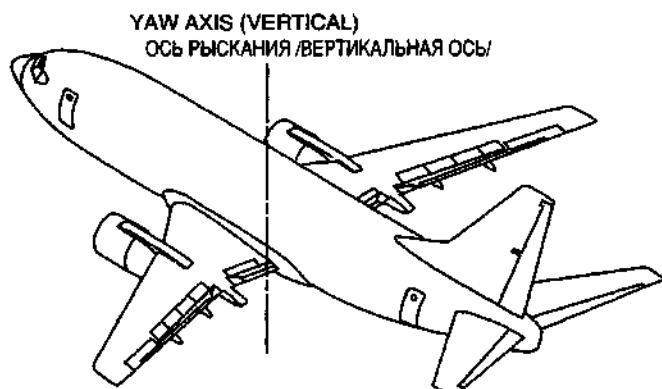
YAW DAMPER, A system that is1 move the rudder a small amount to oppose airplane yaw.
