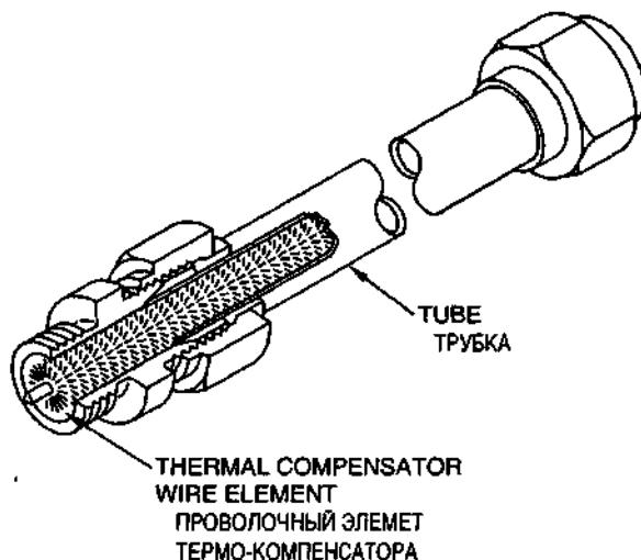
**THERMAL RELIEF VALVE**, A valve which opens to decrease fluid pressure due to high fluid temperature.
