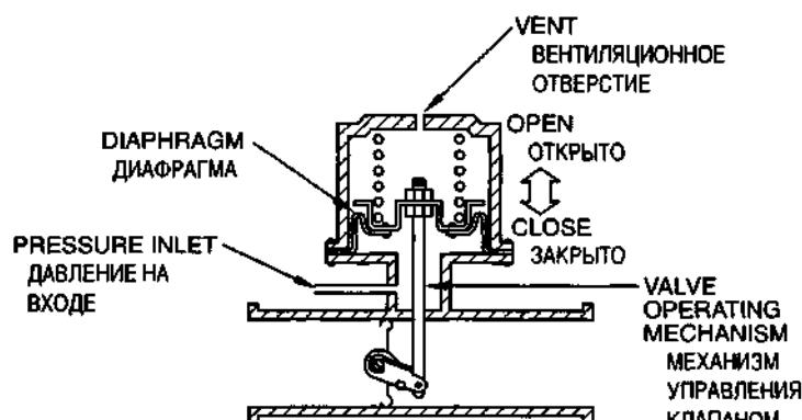
**DIFFERENTIAL PRESSURE**, Pressure relative to another pressure in the same system, measured in pounds per square inch differential (psid).
