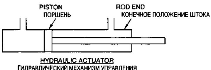
**ROD END (NO. 2)**, A mechanical device usually a bearing, clevis or similar component attached to the end of a link or push-pull type rod.
