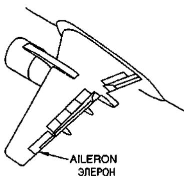
**AILERON FORCE LIMITER**, An electro-mechanical device for limiting the control wheel movement by the autopilot during autopilot operation.
