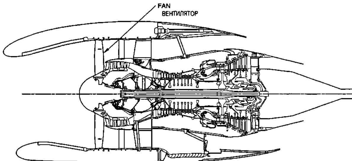
**FAN AIR**, The portion of airflow through a turbofan engine which passes only through the fan.
