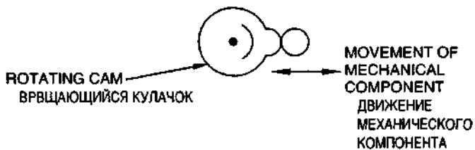
**CAM-OUT**, An autopilot condition in which the actuator detent piston is overridden, either manually or by the other autopilot actuator.
