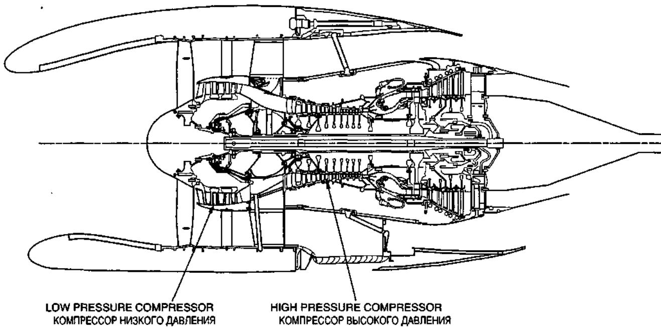
**COMPRESSOR STALL**, An event that occurs when there is a complete stoppage of air or reversal of air flow through the compressor.
