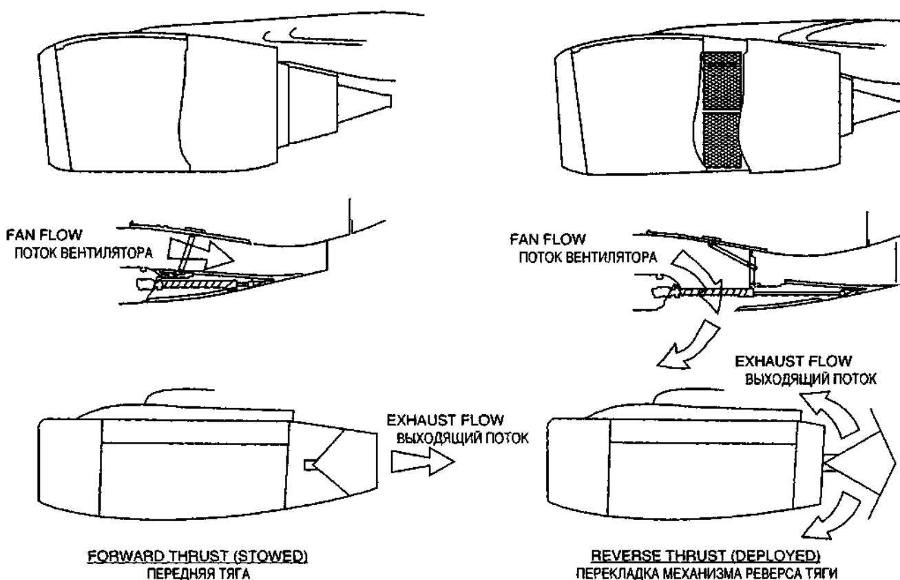
**THRUST REVERSER COWL**, A cover around the thrust reverser of the engine that can be opened to access components for maintenance.
